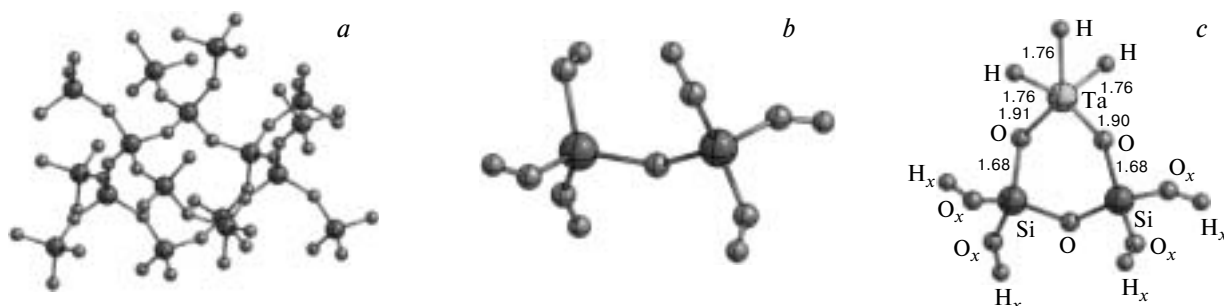
Fig. 1. Structures of \beta -cristobalite (a), the cluster, which models the silica surface (b), and the optimized structure of the (\text{H}_4\text{Si}_2\text{O}_5)\text{O}_2\text{TaH}_3 cluster (c) ( \text{O}_x and \text{H}_x are the fixed atoms). Here and in Fig. 2, the bond lengths are given (in Å).
